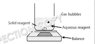
As the reaction pens, gas leaves the beaker and the reading on the balance decomposition  $\mathbf{r}$
