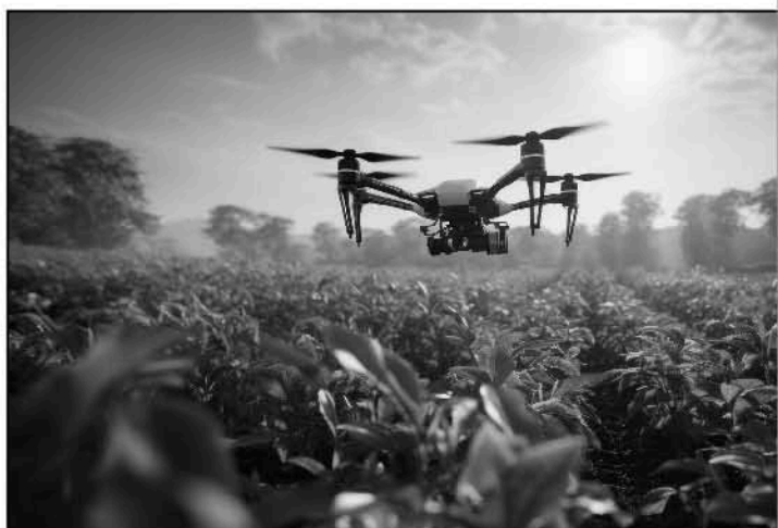
Drones equipped with modified cameras use NIR (Near Infrared) photography to map plantations and monitor plant health effectively.
